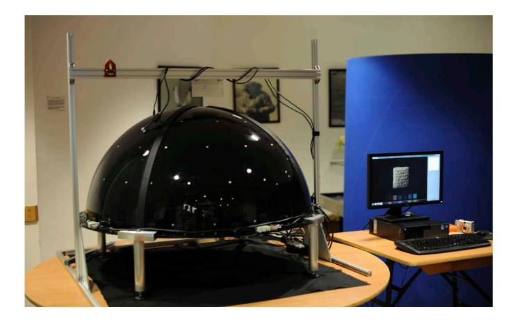
Figure 6: an RTI dome. Courtesy of Graeme Earl Capture surface properties that can be used in supplementary digital synthesis and enhancement of the captured surface using other innovative software (eg through computer graphic modelling).
