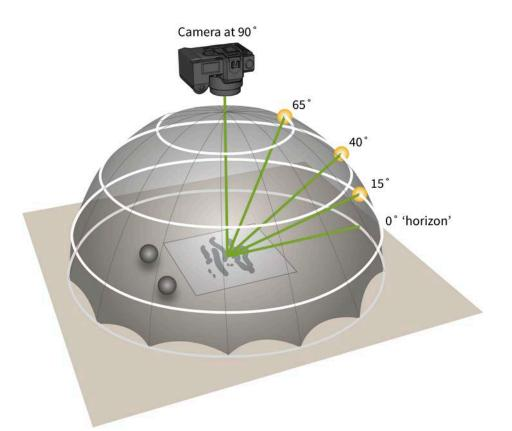
Figure 12: a virtual geodesic lighting dome.
