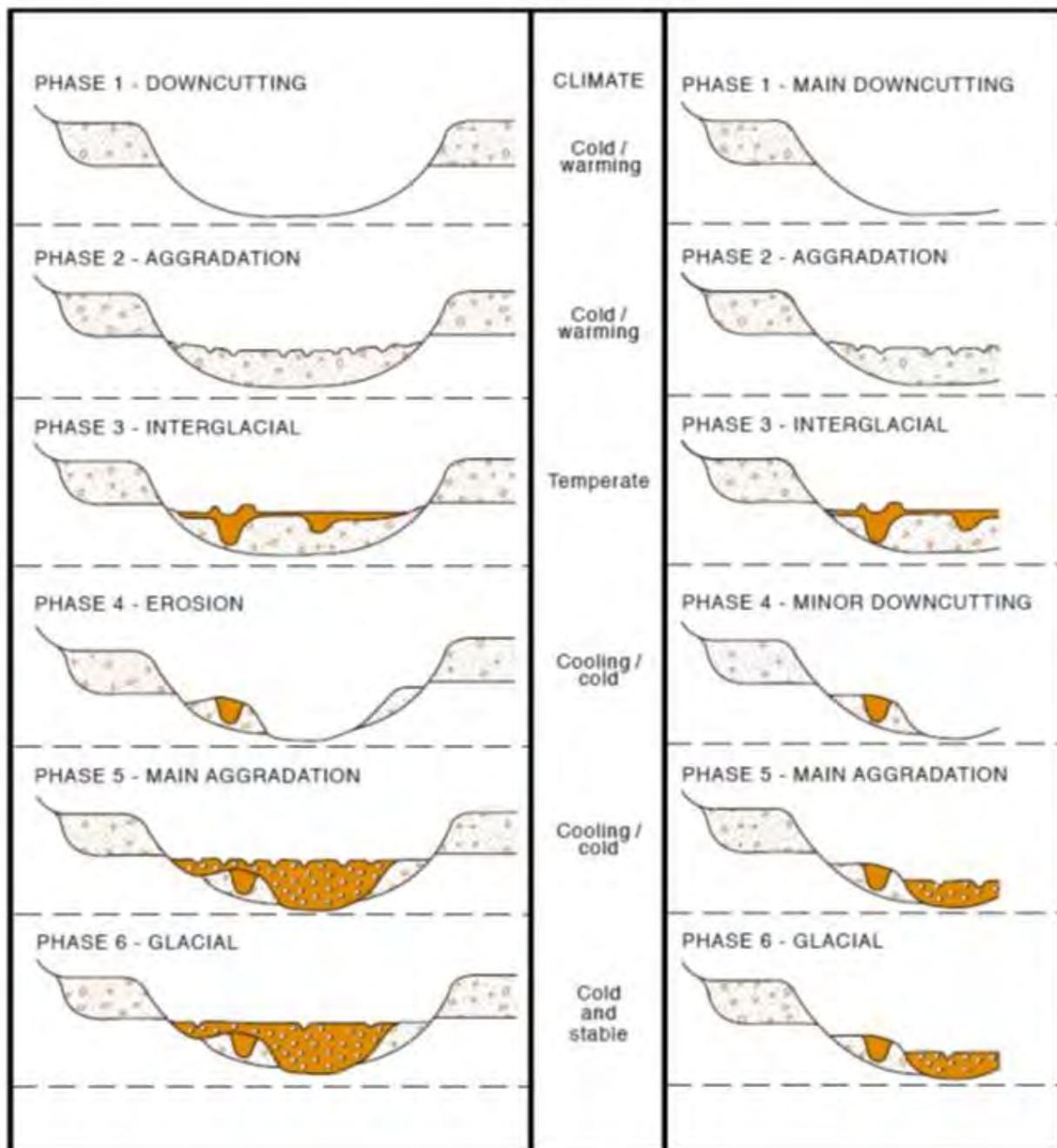
Figure 4. Model of terrace formation in synchrony with glacial-interglacial climatic fluctuation.
