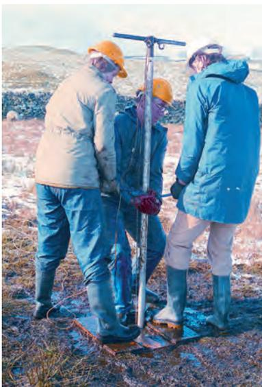
**Fig 6** Using a modified Livingstone piston corer in kettle hole deposits on the A66 at Stainmore, County Durham (photo by J P Huntley).
