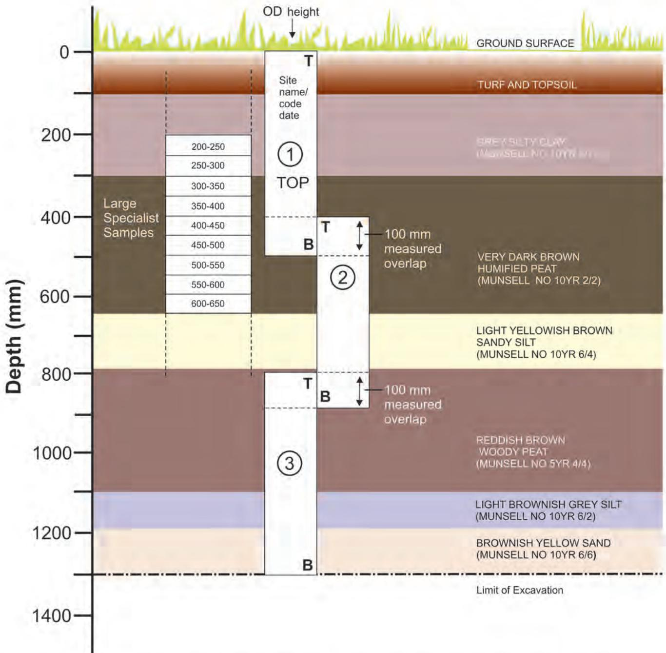
Radiocarbon samples - no thicker than 10mm. Samples for dating can also be taken from vertical monolith or monolith tin placed horizontally. These are sub-sampled in the laboratory as required. Tins in drawing are 500x100x100mm
