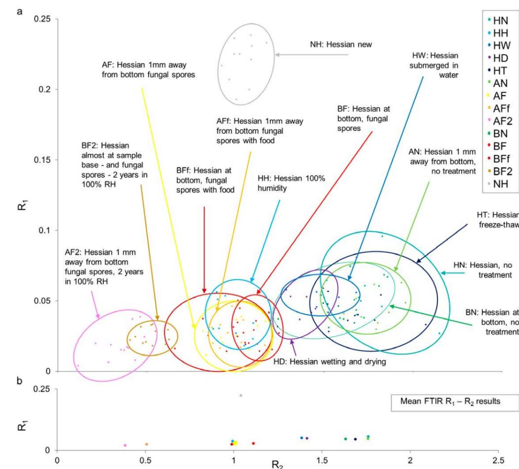
**Figure 3:** Two peak ratios for hessian fibres, termed R1 and R2 are calculated at different moisture contents and following fungal treatment: a) An R1 versus R2 plot distinguishes the different moisture and fungal treatments for at least ten specimens of hessian fibre forming distinctive clusters. b) Mean R1 and R2 values from the sample sets in part a). (Maudrill, Dams *et al.*, 2023).
