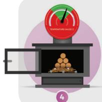
**IGNITION:** During ignition, when the stove controls may be set to a maximum ventilation to get the fire going, there is the potential to lift heavy burning materials, such as paper and card, from the fire box and for it to be ejected from the chimney over the thatch. The use of firelighters and kindling in preference to paper and card will reduce the risk. The wood burning stove should NEVER be used as an incinerator, eg for sensitive paperwork and rubbish.
