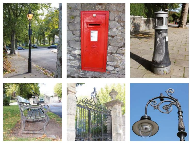
Explore your local area for items made of iron. Much street furniture is made of cast iron. Anything with decoration or lettering forming an integral part of it will almost certainly be cast iron. Decorative wrought iron always consists of thin strips bent, shaped and clasped or welded together at contact points.
