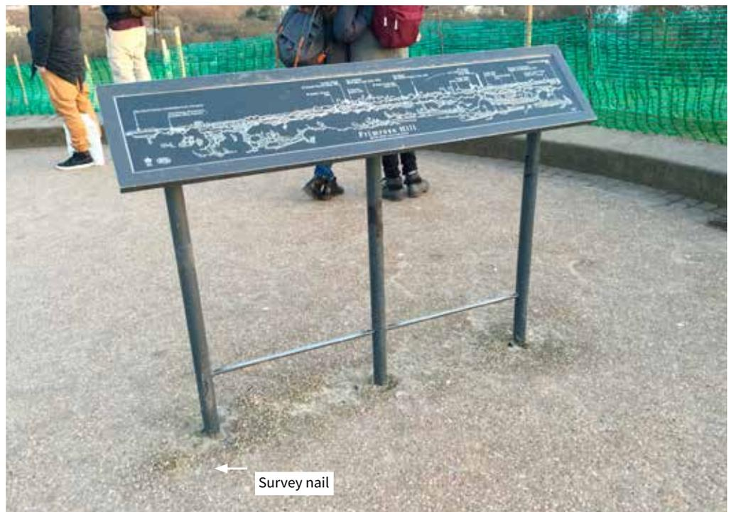
The survey nail near the new orientation panel (right) is about 10.5m away from the real assessment point in the new turf (left).
