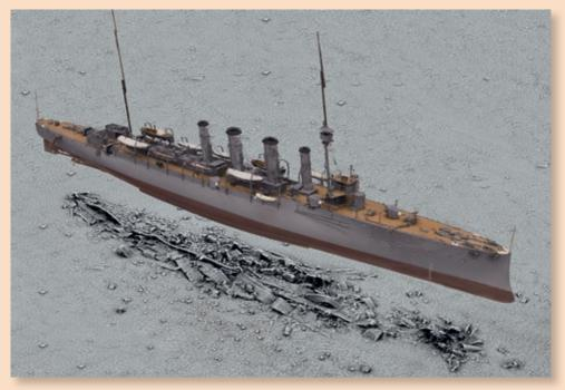
This image shows a 3D scan of the original builder's model of HMS Falmouth in relation to a survey of the wreck on the seabed. 3D scan by Historic England. Access to ship model courtesy of Imperial War Museums. Contains Maritime and Coastguard Agency data © Crown copyright.
