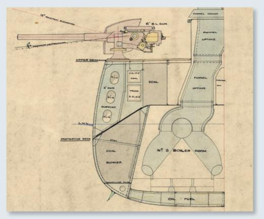
1911 construction drawing of HMS Weymouth, sister ship of HMS Falmouth, showing 6" gun, armoured deck, coal bunkers, tumblehome and V-shaped boiler. © National Maritime Museum, Greenwich, London.
