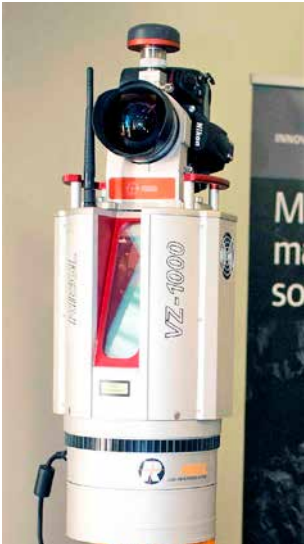
Figure 13 (left) RIEGL VZ-1000 pulse scanner with a mounted Nikon DSLR camera © 3D Laser Mapping Ltd
