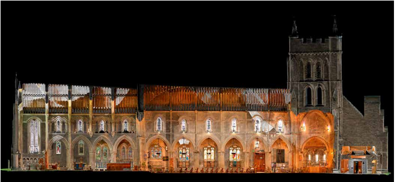
Figure 6 Section through a unified and colourised point cloud of St Hilda's Church, Hartlepool, County Durham © Digital Surveys Ltd
