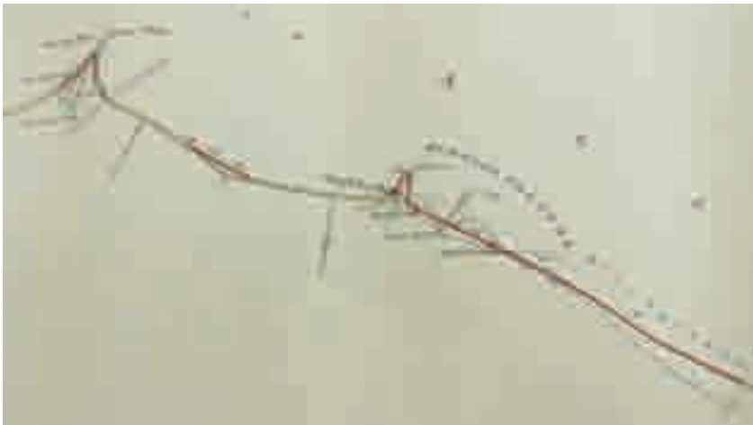
Figure 42 Revised road alignments, drawn in red, for the area around the Garrigill Burn and Ashgill, as proposed in 1823.
