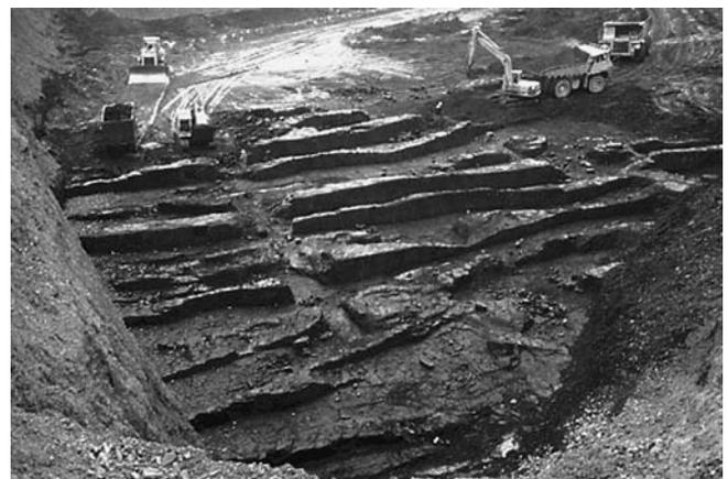
**Fig. 52:** *Later medieval 'pillar and stall' coal mining exposed by modern opencast mining at Coleorton, Leicestershire*
