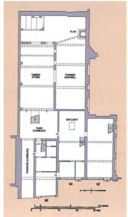
Fig 54 A ground-floor plan of 92–96 Curtain Road in 2002, before the demolition of the rear buildings, a former saw-mill and timber store.
