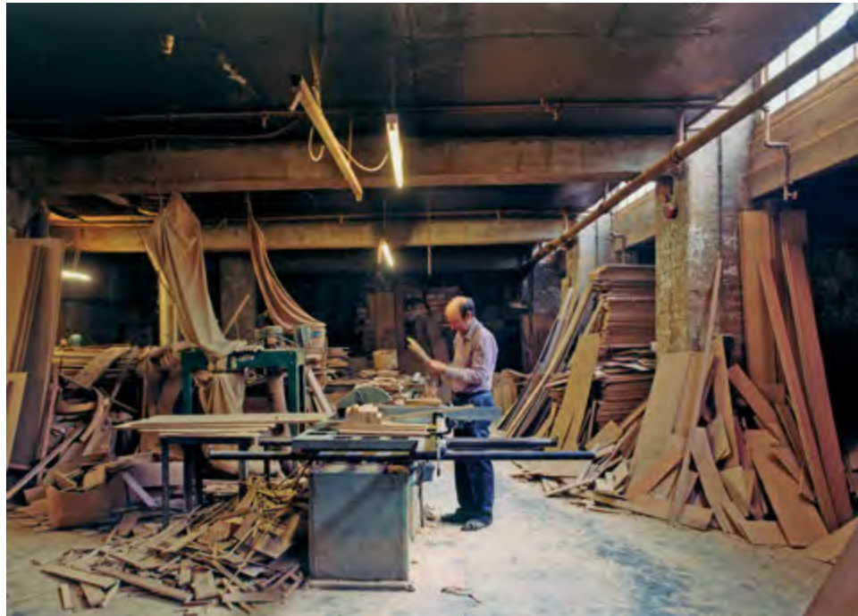
Fig 42 A basement machine shop at 16 Provost Street with Mr Brian Laye operating a table saw. Light from the ground-floor windows is able to reach the basement by canting or splaying the ceiling upwards before it meets the front wall. This feature can be found in manufacturing buildings across the district.
