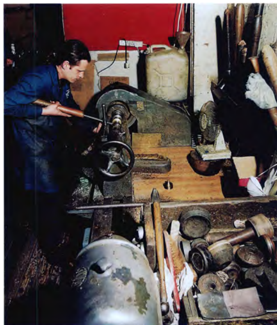
Fig 24 (right) Metal spinning on the ground floor of the W Bayliss & Son (Birmingham) Ltd Works at Nos 4–5 Mary Street. The various wooden-handled tools used for spinning are arranged along the wall behind the lathe. [AA99/087|8]
