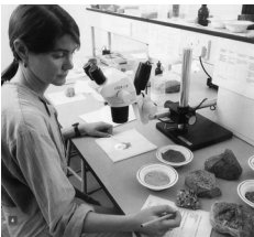
Laboratory analysis of mortar constituents, West Dean College
