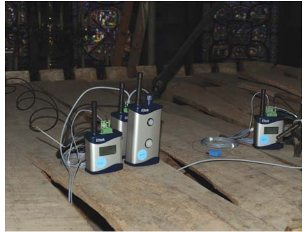
Sensors monitoring relative humidity, temperature, light, UV radiation and movement on the Black Prince's tomb at Canterbury Cathedral. ©Tobit Curteis
