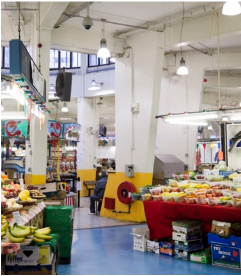
Figure 37 City Market (Arthur Ling, city architect and planning officer, 1956–8). Tapering concrete columns around the central ring lit from the clerestory window. [DP059615]
