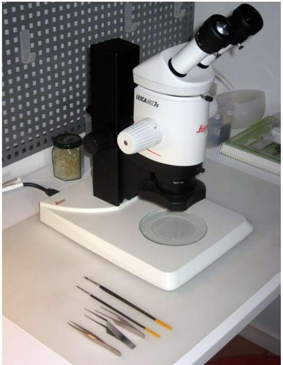
**Fig 2** Handling equipment: left to right, fine 'hard' watchmaker's forceps; two pairs sprung 'soft' forceps; paintbrushes.
