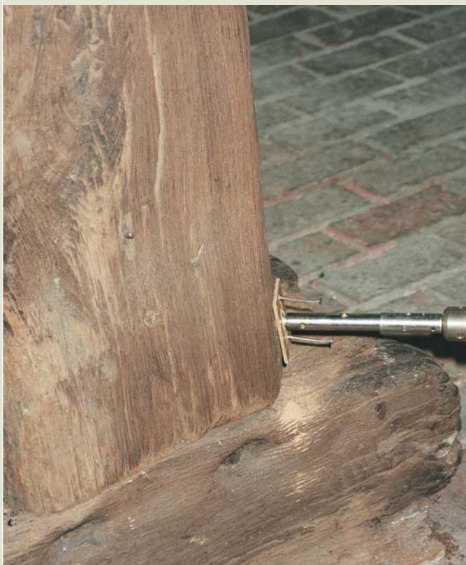
FIG 19 Core being taken at the bottom of a timber so that the resulting hole is less obvious (photo: J Hillam)
