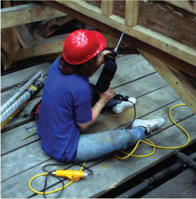
FIG 16 Coring a large tiebeam in the Great Kitchen at Windsor Castle (English Heritage Central Archaeology Service)
