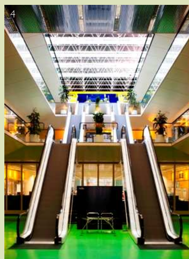
3, 4 The Willis Building, Ipswich 16 Rooftop garden and central atrium, the latter containing the first escalators to be installed in a British office building
