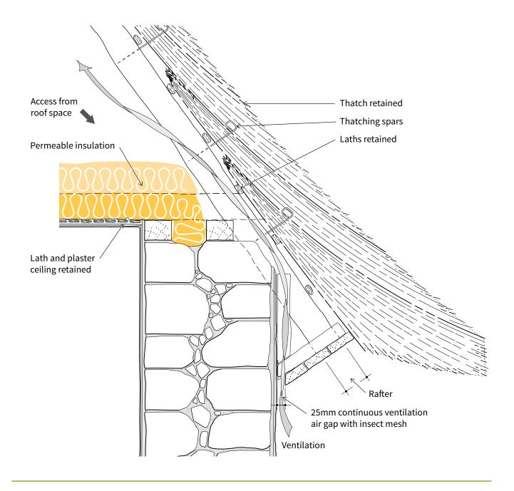
**Figure 10: Cold roof – Roof space insulation at eaves** A conventional cold roof in a thatched building with a clear ventilation path maintained at the eaves.
