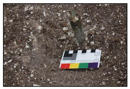
Figure 6: Pitot tube in situ illustrating vertical nature of crash
