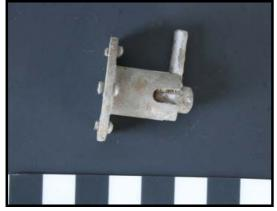
This was one of a number of cowling and panel fasteners that were recovered on the excavation. Several of these still had the original paint scheme adhering to the external face.
