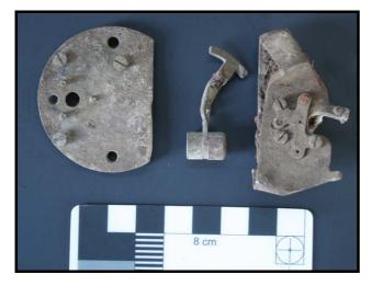
The remnants of the cockpit clock were broken into three individual components. The face, hands and mechanism have not survived.
