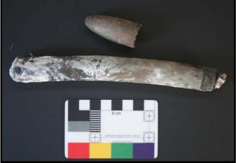
The Pitot tube was present in the port wing of the Mk1a Spitfire and wa used to measure air speed. Its *in situ* presence on the excavation enabled the team to precisely demarcate the area of the airframe and also illustrated the vertical nature of the crash.
