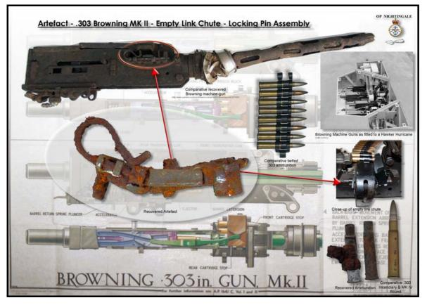
Figure 15: Position of the Browning component from the excavation in relation to the overall gun assemblage. © Mark Khan
