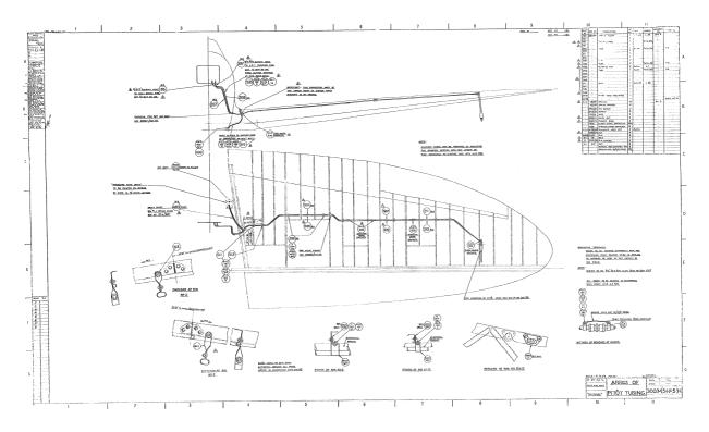
Figure 7: Original Blueprint drawing of the Mk1 Spitfire illustrating position of pitot tube (from Dominic Berry)
