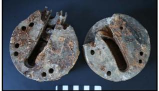
The milled sides of these two artefacts had impacted (and left a cross-hatched indentation) upon the remnants of the spinner of the propeller unit which was painted black.
