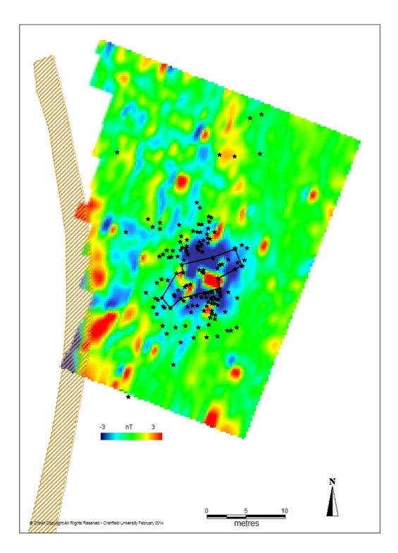
Figure 17: Magnetometer survey results of P9503UP with the excavation trench superimposed, and outlying stray finds marked as stars. Note the darker area of the crater with high central reading of engine components. © Peter Masters
