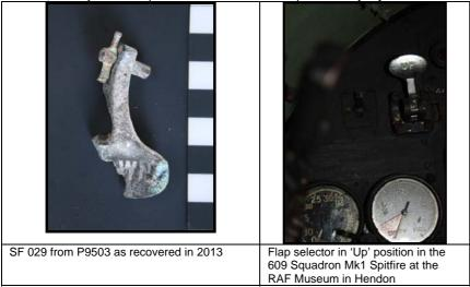
The flap selector is situated in the lower left section of the instrumentation panel of the Spitfire.
