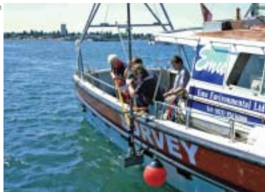
Wessex Archaeology ALSF "Wrecks on the Seabed" project team deploying a Reson multibeam 8125 sonar head from EMU Surveyor
