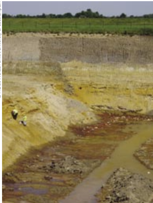
Above: Four OSL dating samples being taken from strata of a varied fluvial sand deposit, Tattershall Thorpe gravel pit (RMC), Lincolnshire a site visited as part of the Trent Catchment project
