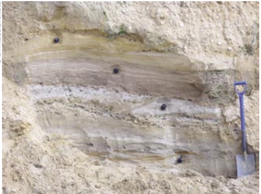
Above: Four OSL dating samples being taken from strata of a varied fluvial sand deposit, Tattershall Thorpe gravel pit (RMC), Lincolnshire a site visited as part of the Trent Catchment project
