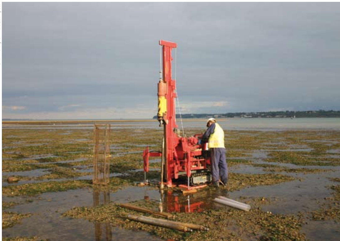
Terrier drilling at low tide at Lepe, Hampshire undertaken as part of the Sussex/Hampshire Coastal Corridor project. Sampling here has, for the first time, revealed the presence of early interglacial deposits beneath the well known estuarine sequences
