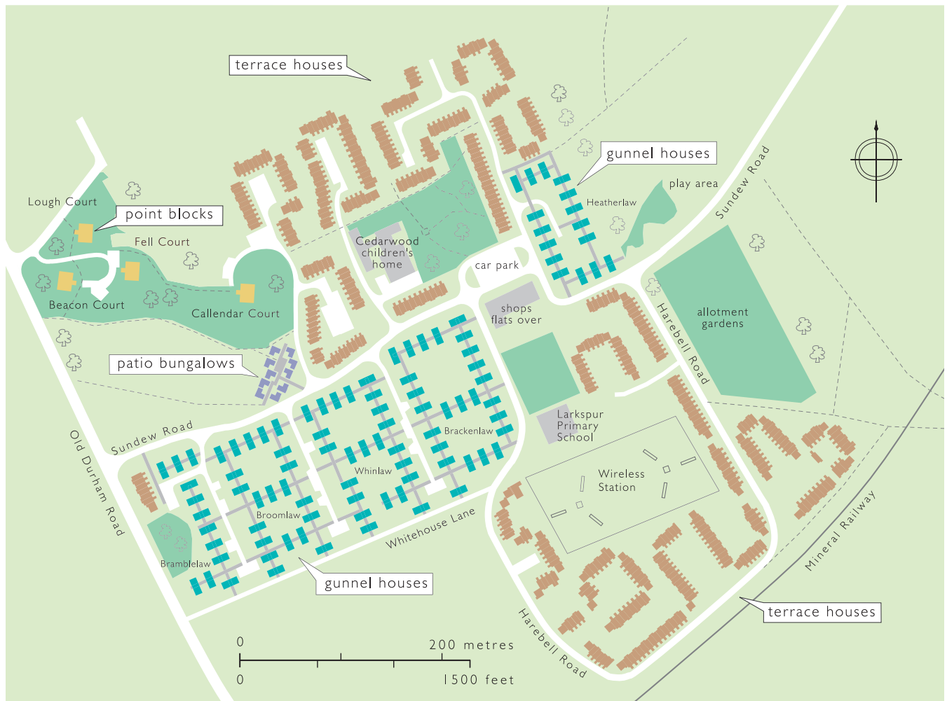
Fig 61 Plan of Beacon Lough East. The estate, which was built in the years 1965–7, mixed low-rise semi-detached and terrace housing with four point blocks and a number of aged persons' bungalows. It was described as a 'safe estate' because vehicle and pedestrian circulation routes were segregated.
