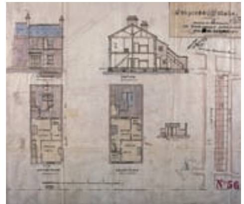
Fig 40 Plans for a row of Tyneside flats on the south side of Ripon Street (on the Shipcote Estate) for George Lucas, dated 1876. The ground-floor plan shows outdoor WCs, a great improvement on the ash closets provided for most flats at the time. [TWAS/T311/56/1876, reproduced by permission of the Chief Archivist, Tyne & Wear Archives Service; AA040377]
