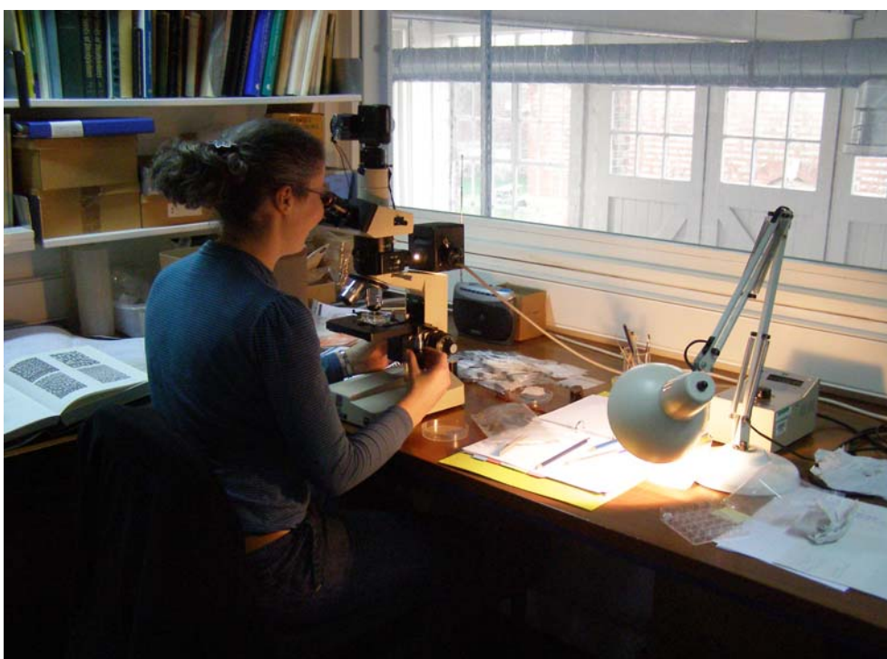
Analysing wood charcoal fragments from the southern hypocaust furnace and sorting them according to species where possible.
