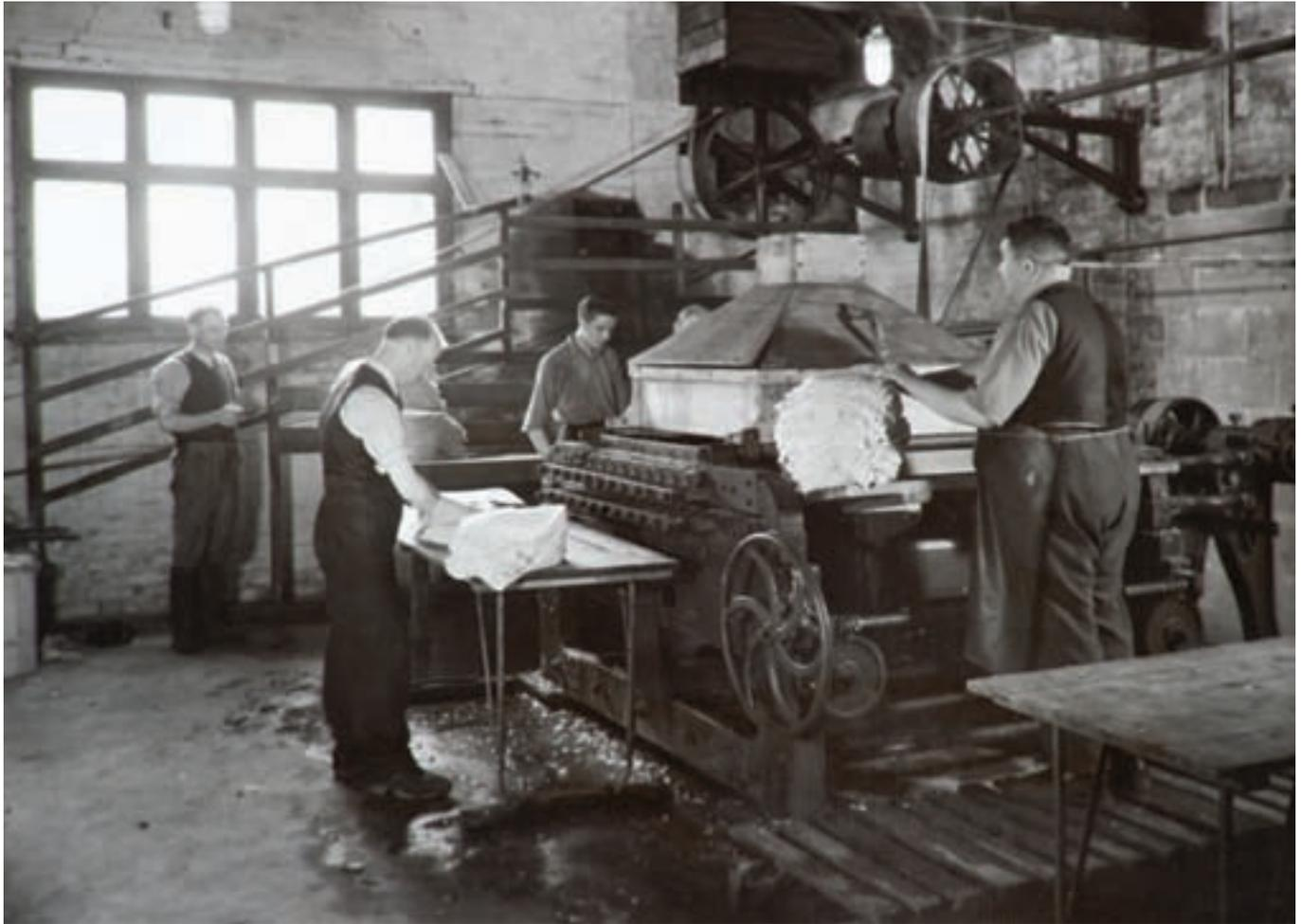
of production from there onwards is very much the same as in straw-hat manufacture – after being steamed the hoods are blocked into shape, stiffened if required and left to dry before being lined and trimmed.
