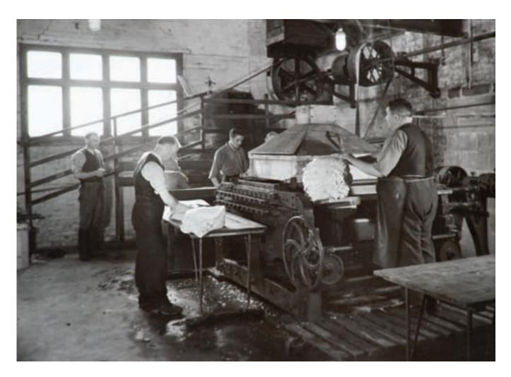
of production from there onwards is very much the same as in straw-hat manufacture – after being steamed the hoods are blocked into shape, stiffened if required and left to dry before being lined and trimmed.
