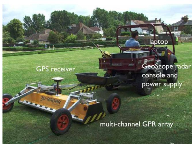
GeoScope three-dimensional ground-penetrating radar survey, utilising a 21-channel towed antenna array.
