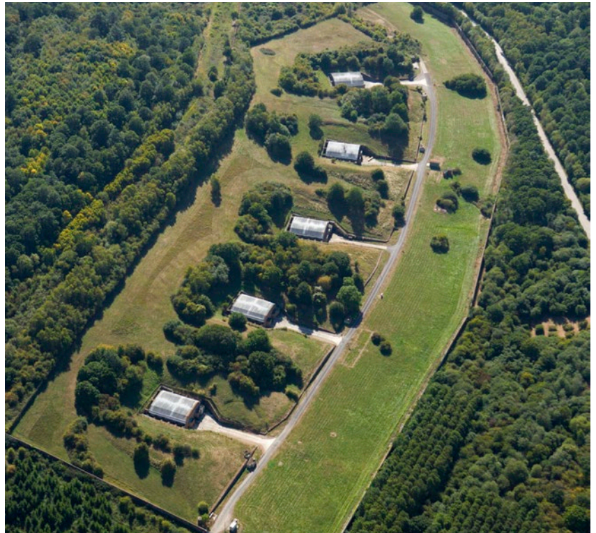
Figure 47 The naval magazines at Chattenden. Each magazine could hold 4,000 barrels of gunpowder and was set within a substantial earthwork traverse. 32 Situated approximately 2km from the Medway, they and the nearby Lodge Hill depot were connected to Upnor by a railway. [26475/032]
