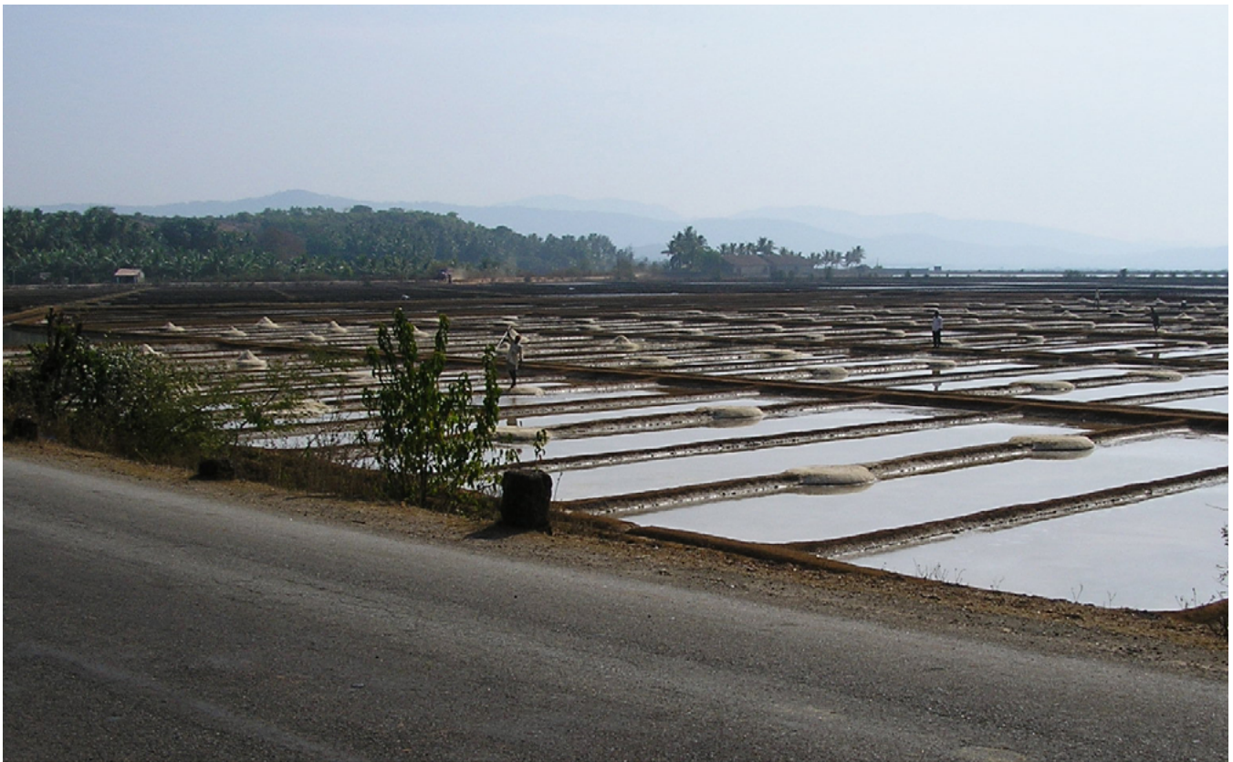
Figure 1 A solar evaporation system, or salina, in operation near Udapi on the Malabar coast, southern India.
