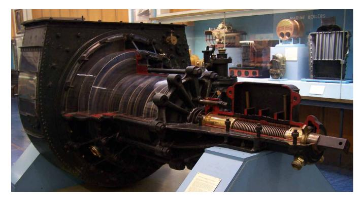
Radial flow turbine engine of the Turbinia, launched 1894, the world's first steam turbine driven vessel. On
