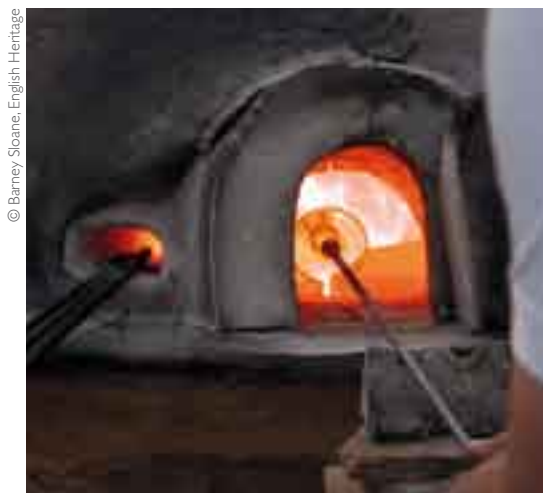
Experimental Roman glass furnace in action reconstruction
