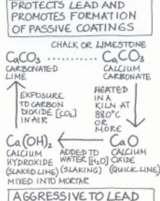
Figure 11 The lime cycle. Calcium carbonate – CaCO<sub>3</sub> – the start and end point of the cycle, is nearly neutral, does not attack lead and can help to protect it. Slaked lime – Ca(OH)<sub>2</sub> – is alkaline and aggressive to lead.
