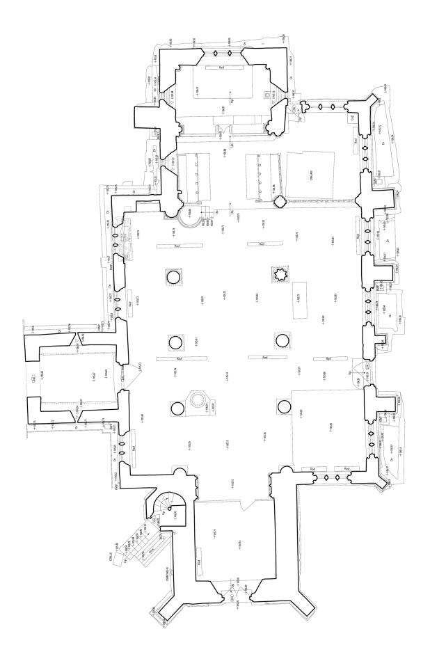
Figure 5.2: Plan showing use of line weights. Originally prepared for presentation at 1:50 scale.
