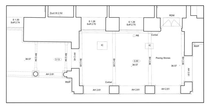
Figure 5.5: Examples of overhead detail; (top) plan with a vaulted ceiling – 1:20 level of detail; (bottom) overhead beams on a plan – 1:50 level of detail.
