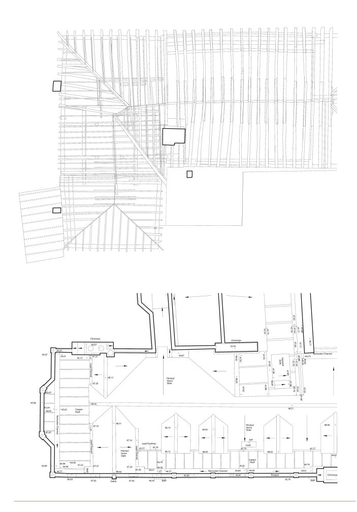
Figure 5.7: Roof plans: (top) example of plan with cover off; (bottom) example of plan with cover on.
