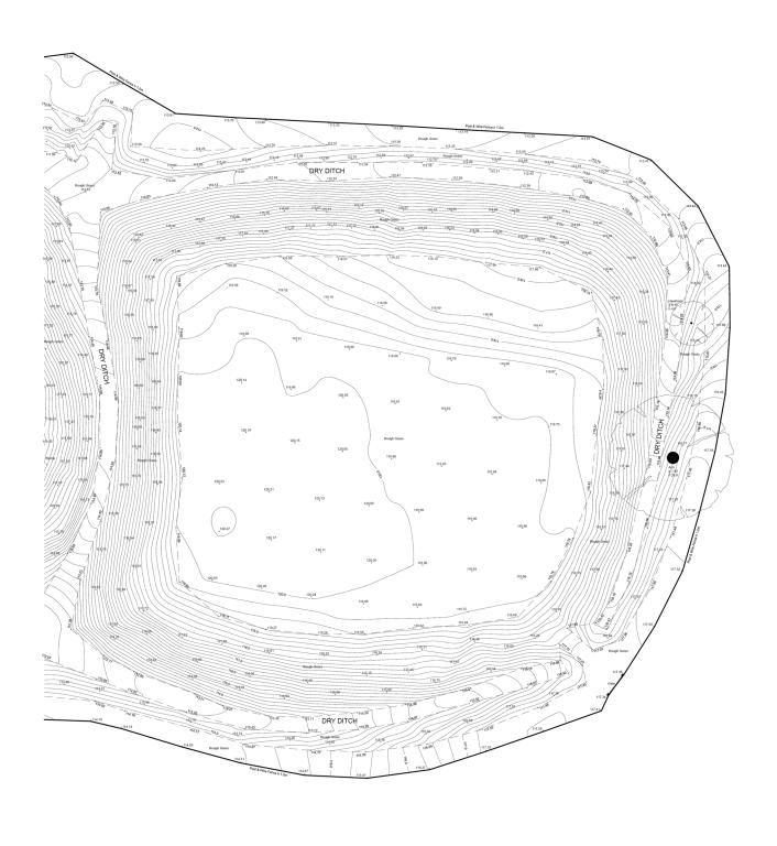
Figure 6.5: Contours generated from a DTM and breaklines. Originally prepared for presentation at 1:200 scale.
