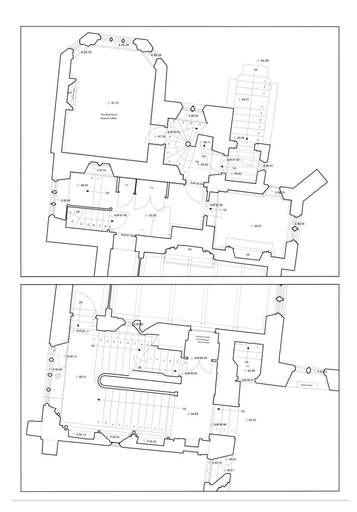
**Figure 5.6:** Two examples of the treatment of staircases on plans.
