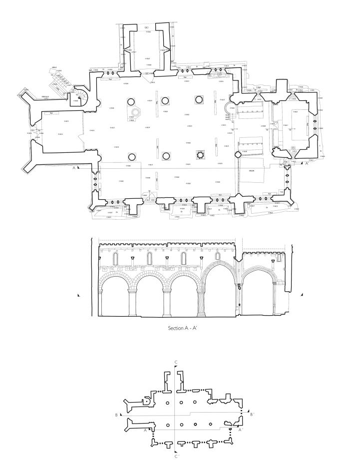
Figure 5.4: (top) Section lines; (middle) shown related to plan: (bottom) multiple sections depicted on a key plan.
