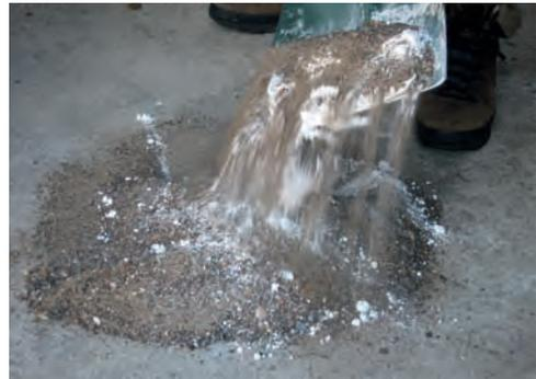
*"Hydraulic limes should be left (after being wetted and covered up) for a period varying from twelve to forty-eight hours, according to the extent of the hydraulic properties they possess; the greater these are, the longer will they be in slaking... Only so much should be slaked at once as can be worked off within the next eight or ten days."*
