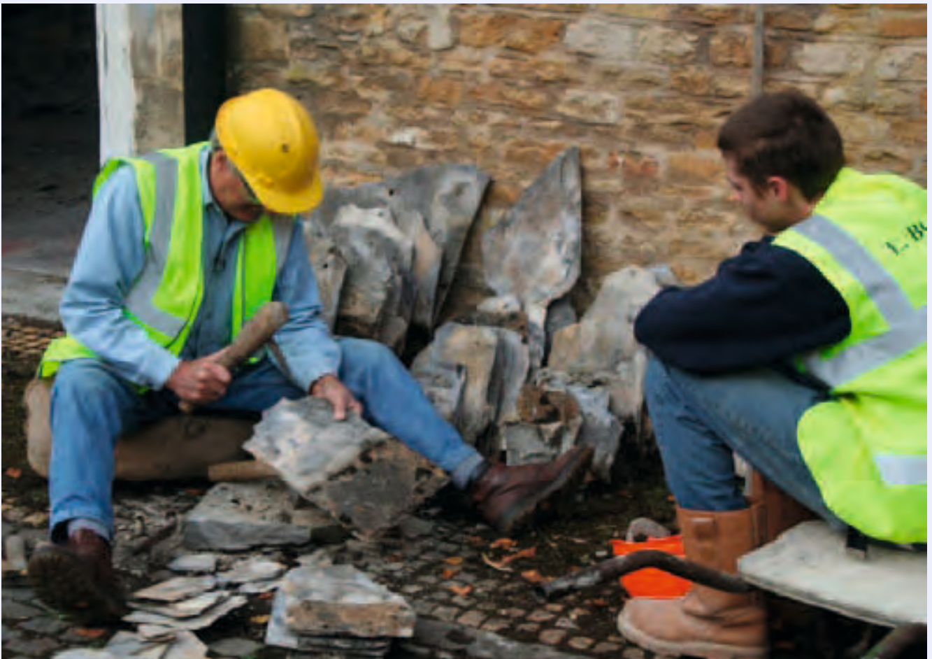
David Ellis making Collyweston slates. There are currently no reliable sources of good quality Collyweston slate. Nearly all the material used for repair and conservation is now reclaimed from other buildings, which is not sustainable in the long-term. (2D5). © Chris Wood, English Heritage
