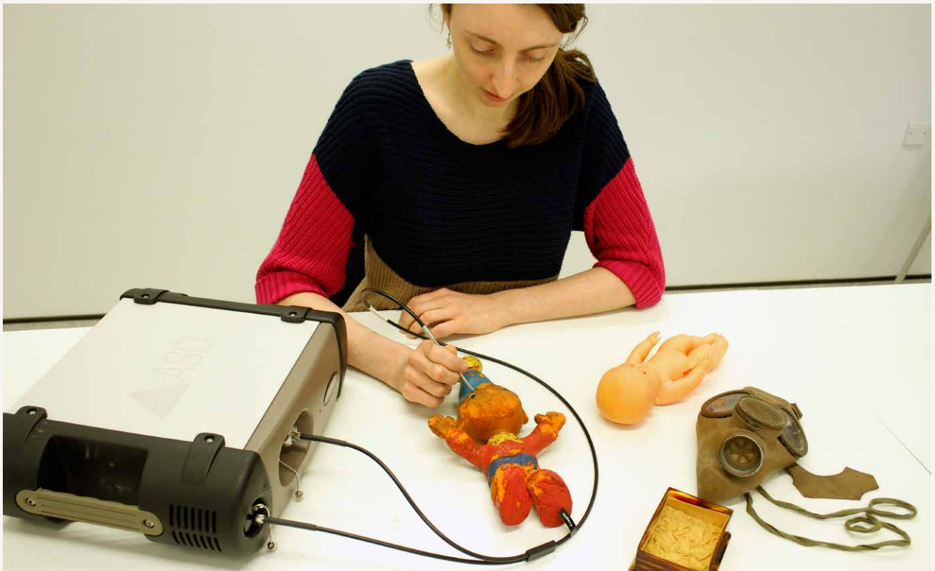
Near infra-red spectroscopy being used to identify the plastic in a modern doll during the Heritage Smells Project. Similar analysis has been undertaken on modern collections at Brodsworth Hall, Dover Secret Wartime Tunnels and York ROC bunker (2C2). © University College London
