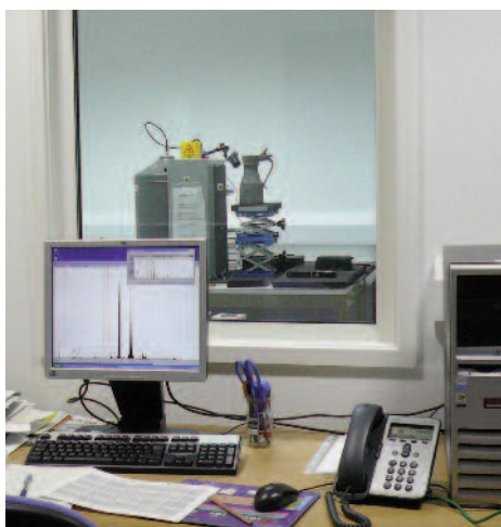
Figure 32 Custom built air-path XRF being used [at NMS] for non-destructive examination of a Scottish "tappit hen" pewter flagon. © Trustees National Museums Scotland
