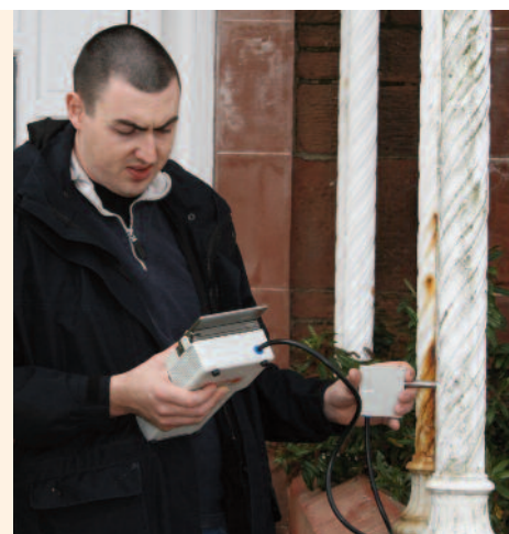
Figure 34 Craig Kennedy undertaking hand-held Raman spectroscopy to analyse the paint on the surface of a cast iron canopy in Rothesay, Bute, Crown Copyright, Photo: Alan Simpson
