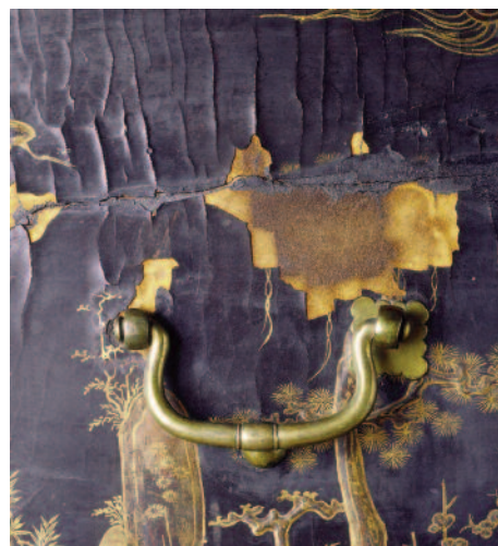
Figure 15 RH damage to a lacquered chest at Belton House, Lincolnshire. A low RH caused the materials to dry and crack. ©NTPL/Rob Matheson
