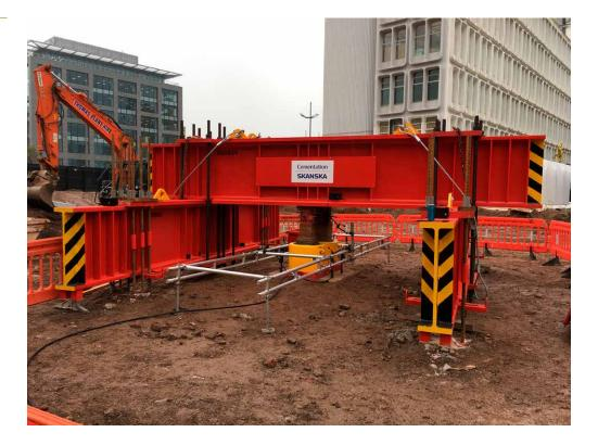
Figure 28: Static load test. © Cementation Foundations Skanska
