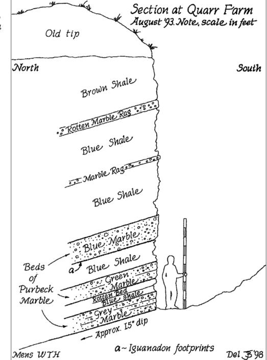
Despite its name, Purbeck Marble is a sedimentary rock and not a true metamorphic marble. Classified as a biomicrudite limestone, Purbeck Marble is a dense stone with low porosity (less than five per cent), low absorption and high compressive strength (over 100 MPa) perpendicular to the natural bed.
