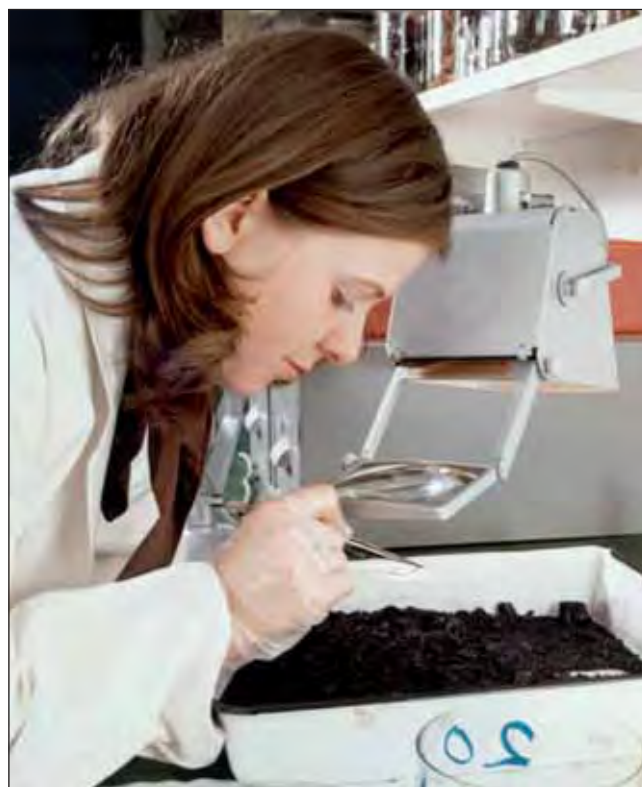
Fig 16. Removing rootlets from a sample of charcoal for conventional radiocarbon dating at AERE Harwell. (© NDA)
