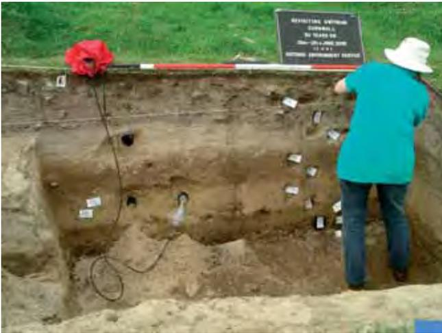
**Fig 4** Taking measurements of radiation dose by gamma spectrometry for OSL dating at Gwithian, Cornwall (© Dr H Roberts, Aberystwyth University)
