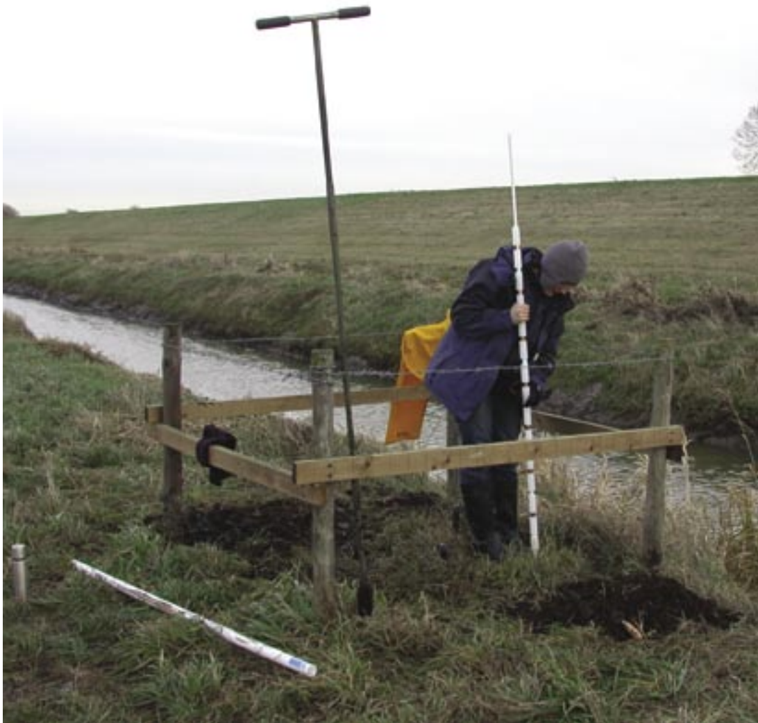
Fig 2 (left). Installing samples of experimental materials at Fiskerton, adjacent to the north delph of the River Witham. A rod of copper samples is being placed in an augered hole
