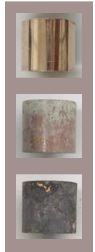
Fig 3. Copper samples: before burial (top); from an oxidising horizon (centre); and from an anoxic and reducing horizon (lower)
