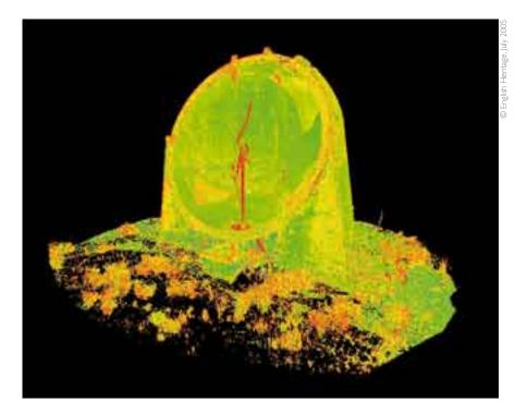
Point cloud data captured by terrestrial laser scanner for the 30ft Reflector
