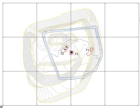
was added to the stack using heavier plant and compacted using a self-propelled vibratory roller. The soil was compacted in 150mm spits and this methodology continued until the maximum height of the stack was reached, at 8.9m.
