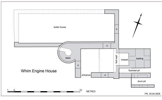
Plan of an engine house at the Buckfastleigh mines. Though the structure is now collapsed, enough remains to interpret its function as a winding or 'whim' house used to hoist material in a nearby shaft
