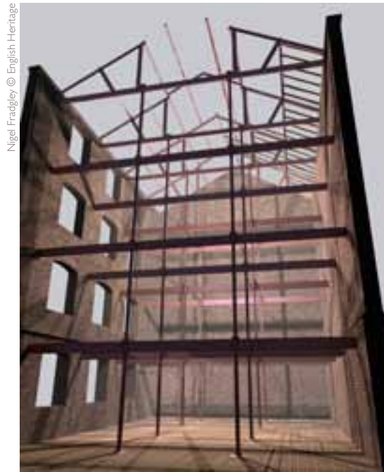
Reconstruction of the iron frame of the wing, as it was rebuilt following a fire in 1811
