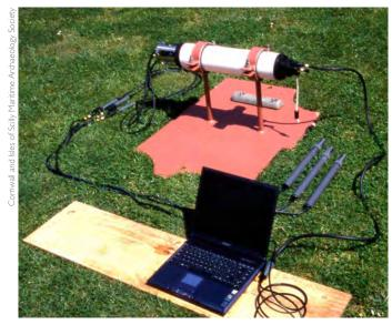
A sub-sea data logger ready to be installed on the protected site of HMS *Colossus*, Isles of Scilly, so as to remotely collect environmental data.
