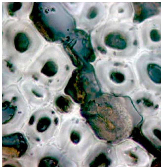
Figure 39 Scanning electron microscopy (SEM) image of elm wood cells showing cavities distinctive of soft-rot fungal attack, developed during prolonged storage in tap water (magnification \times 1,000 ).
