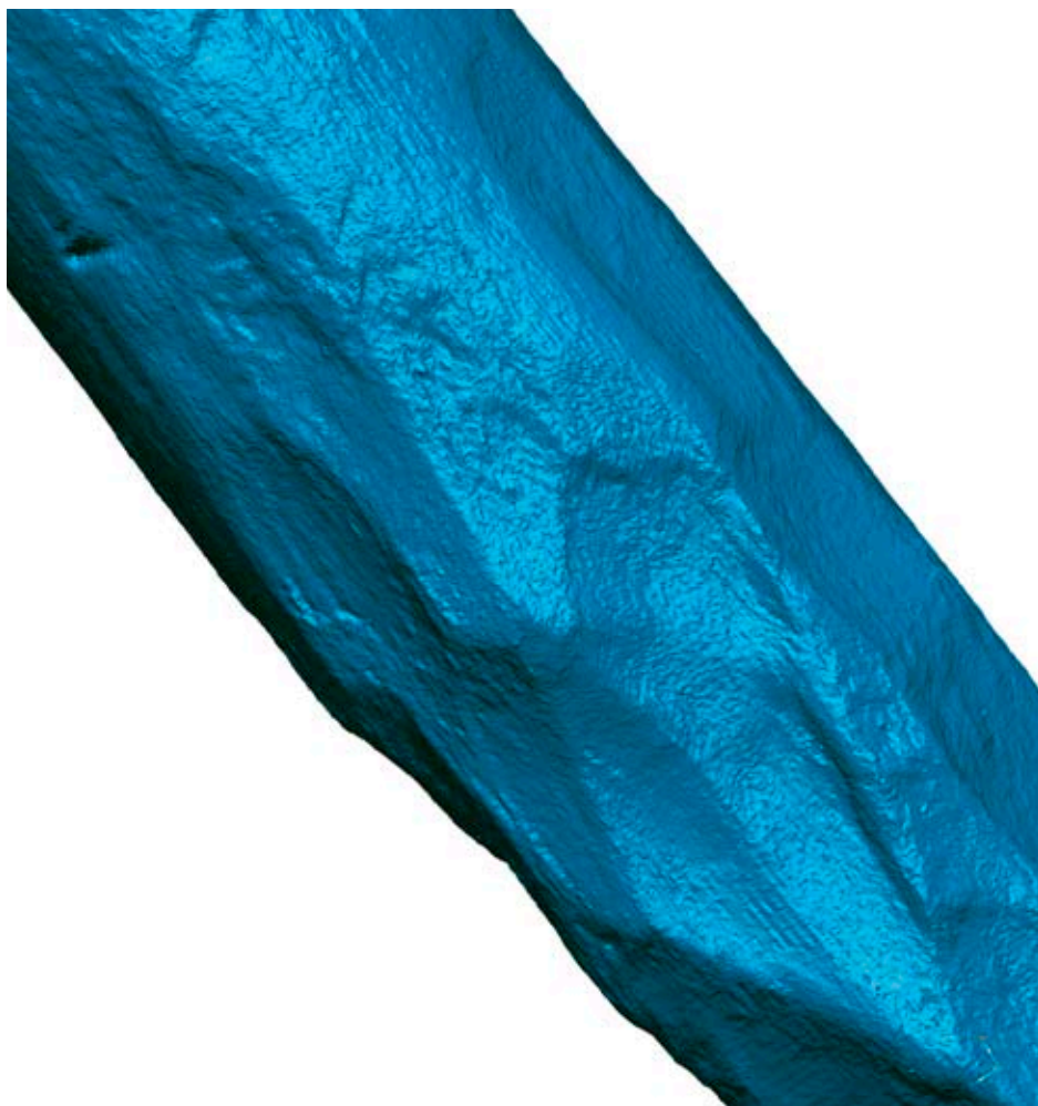
Fig 23 Laser-scanned image of cut wood enabling detailed comparison of tool signatures to be made (© Birmingham Archaeo-Environmental and VISTA).
