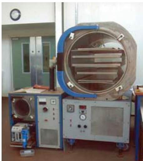
Fig 46 Large vacuum freeze-dryer.
