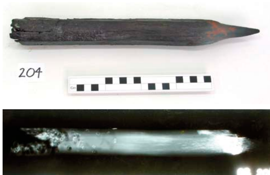
Figs 44 and 45 Wooden pike shaft from an Elizabethan shipwreck, which in the top image appears to be in a sound condition, while the X-ray image reveals the extent of the mollusc damage at one end and the high concentration of iron salts from the iron socket at the other end. © University College London.
