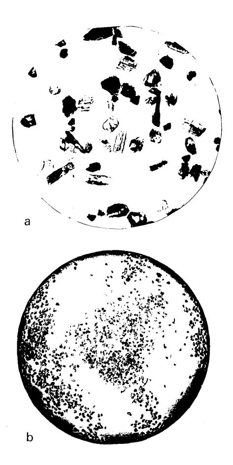
Plates: heavy mineral photomicrographs of Bii (a= x65) and Biv (b= x45) amphorae (N. Bradford)
